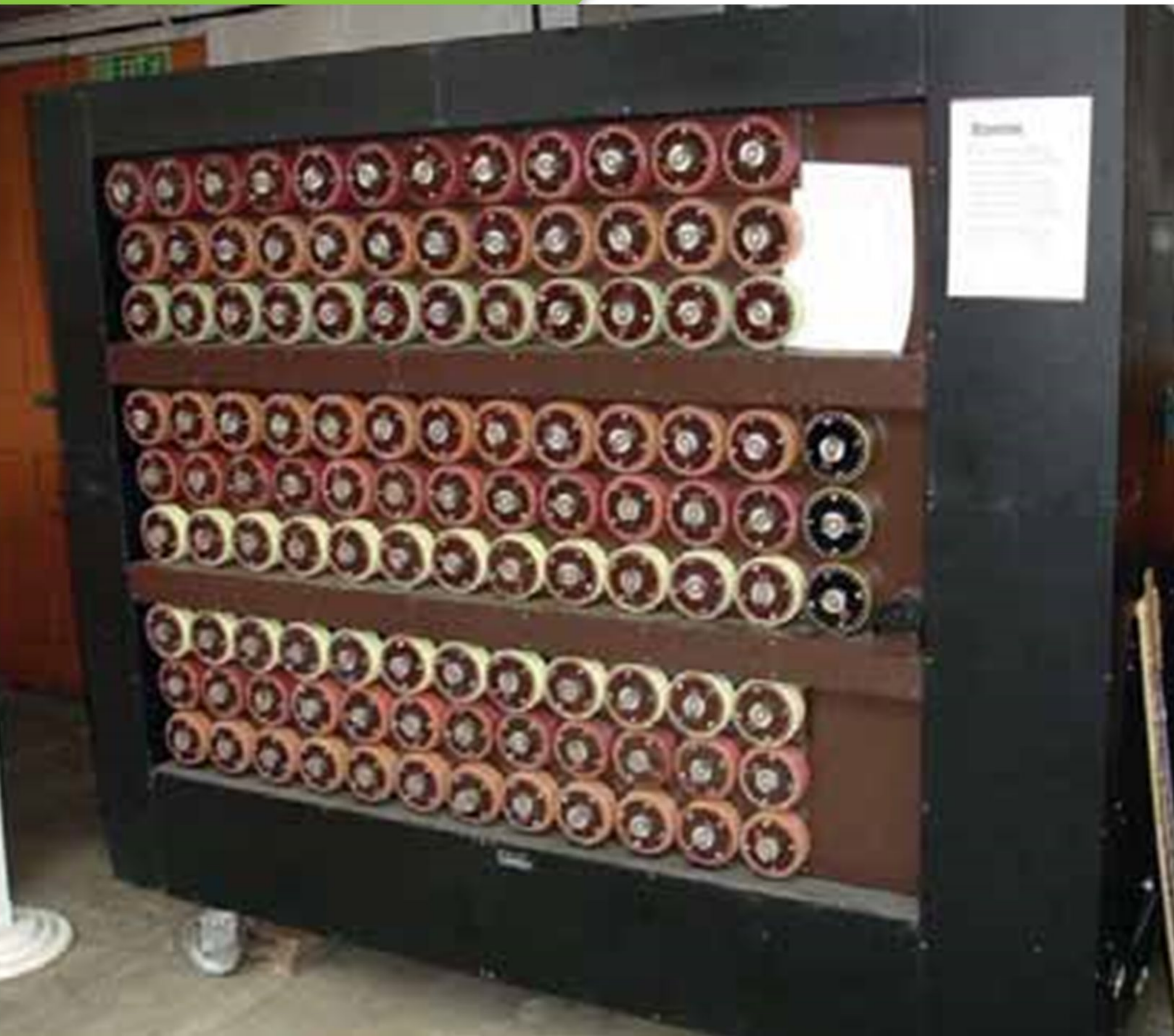
■ Figure 3.21 A reproduction of the machine used to break the Enigma Code during the Second World War, the subject of the novel Enigma by Robert Harris
